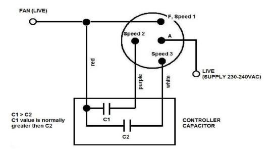
Fig.9 Rotary switch and controller capacitor wiring diagram.
